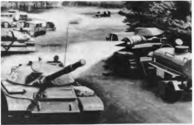
Figure 6-65. Vehicle decontamination. The TMS-65 can decontaminate vehicles in the field by spraying decontaminating agents through a jet exhaust; a tank can be treated in about three minutes.
